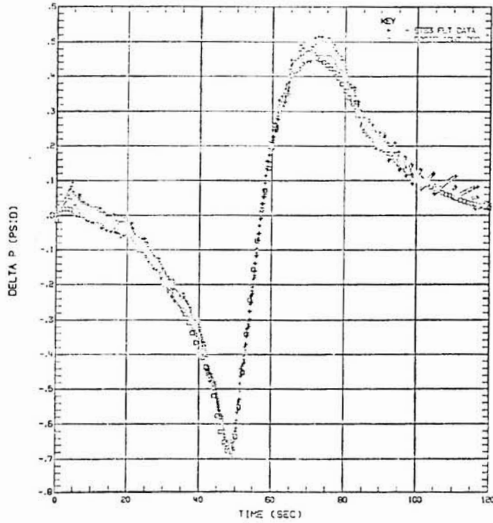
Figure 18.- STS-3 ascent correlation results. OMS pod to ambient differential pressure.
