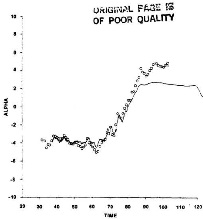
(c) Angle of attack (ALPHA) versus time from lift-off.
